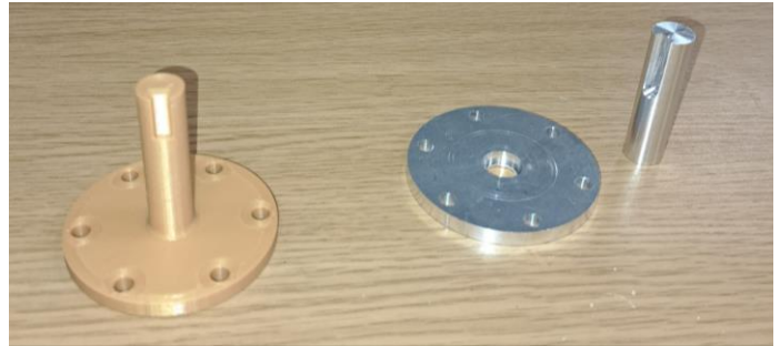
Fig. 13. Plastic Custom Shaft (Left) and Aluminum Shaft (Right)
