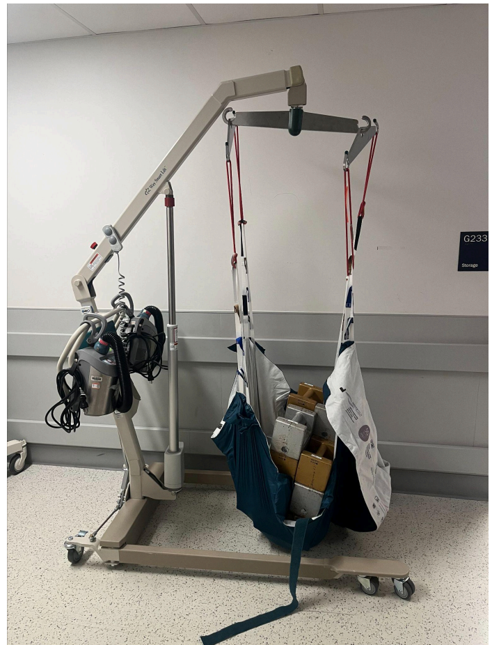
Fig. 5. Hoversling Repositioning Sheet and Prusik Rope Holding 950 lbs. off the ground. This figure depicts the testing apparatus and loop connector replacement accommodating as much weight as the UVA hospital could provide for testing.
