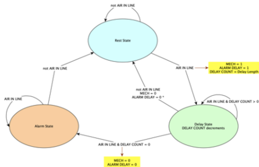
Figure 2: Finite State Diagram of Device Functionality
