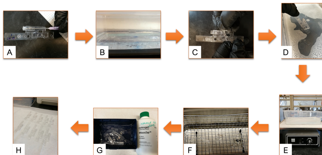
Figure 4-3. Outline of cartridge recycling protocol. (A) depicts ball removal. After adhesive is pierced, moderate force is required to expel the insert from the inlet. (B) shows a lateral view of chips submerged in IPA. (C) shows the removal of polymeric adhesive from the cartridge. (D) illustrates the submersion of the cartridge in soap solution after removal of polymeric adhesive and residue. (E) shows the cartridges in soap solution as rotation occurs. (F) This image shows submerged cartridges in the sonication basket. (G) shows submersion in RNase Decontamination Solution. (H) Sterilized chips as arranged before the drying step.
