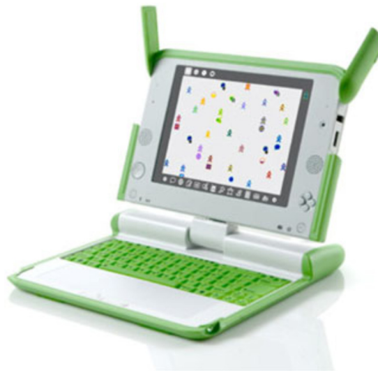
Figure 3: The XO Laptop. This is the laptop OLPC provides the participating schools. Built with students in mind, this laptop is waterproof and shock resistant. (Meza-Cordero, 2016, p.9)
