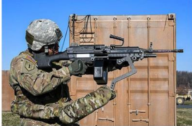
Figure 2: Army Sgt. Michael Zamora uses a prototype Third Arm exoskeleton to easily aim an 18-pound M249 light machine gun during testing at Aberdeen Proving Ground, Maryland, on March 14, 2018. (U.S. Army photo by Conrad Johnson) (Cox 2018)
