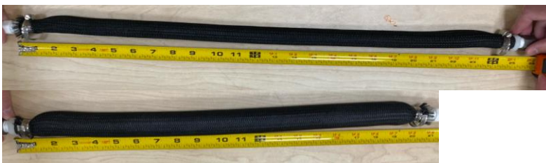
Fig. 19. Muscle two contraction testing. 24.5” resting (top) and 20” after contraction (bottom).
