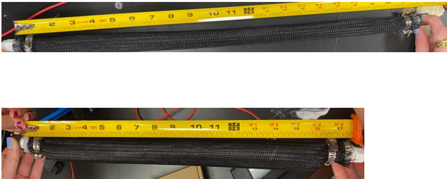
Fig. 18. Muscle one contraction testing. 21” resting (top) and 16.75” at maximum contraction (bottom).
