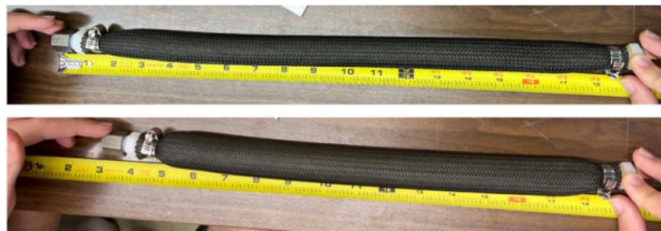
Fig. 11. Change of length test of a McKibben muscle conducted by the 2022 Capstone team (Applegate et al., 2022).
