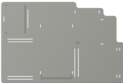
Fig. 10. Electronics housing board. This is designed to hold a full length breadboard, air pump, solenoid, Arduino, and a relay board.
