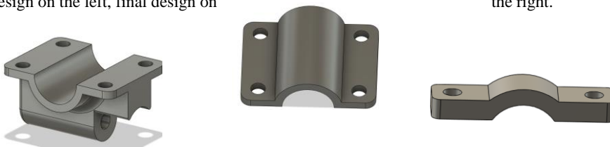
Fig. 6. Muscle hinge and clamp designs. The image on the left and center were muscle clamps that were used in the initial design, when the muscle clamps could rotate at the end of the lever.
