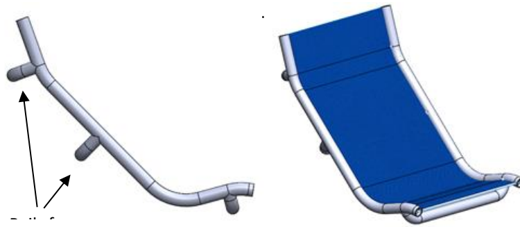
Fig. 1.9. Initial seat design. This would attach to the central pipe of the frame. View (a) shows a profile view of the seat with attachment rails; view (b) shows an isometric view of the seat.
