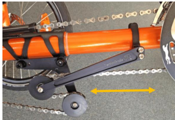
Fig. 1.8: Chain gobbler on a tadpole trike. Each idler wheel is fixed to their respective parts of the telescoping arm. As the arm changes in length, so does the distance between the idler wheels. As a result, the chain remains taut for any length of the arm (Catbike Boom Adjust Chain Tensioner, 2018).
