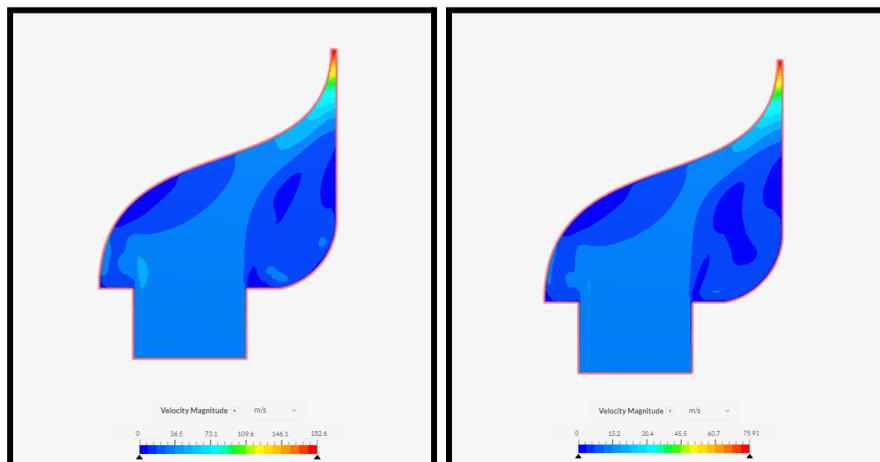
**Figure 6: CFD analysis of final internal flue shape.**
