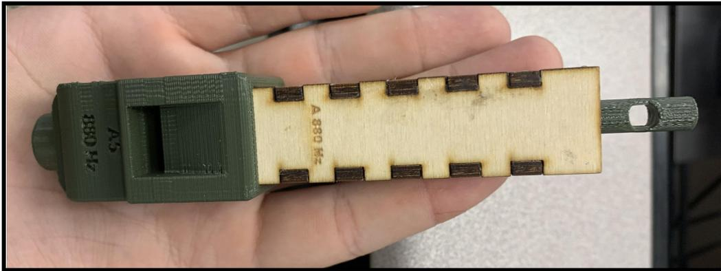
**Figure 8: Image showing final assembled A5 880 Hz pipe.**
