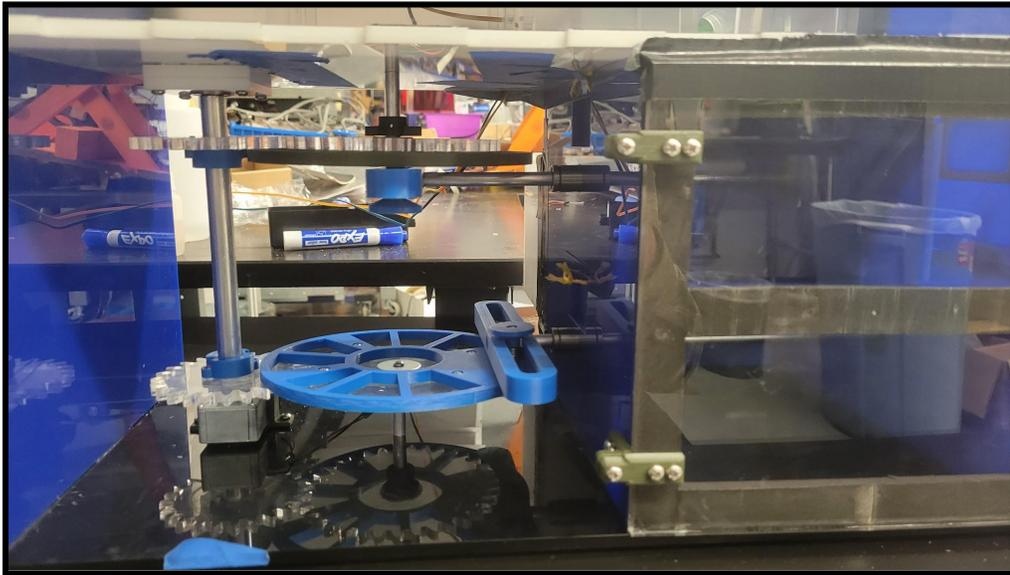
**Figure 12: Picture of the bellows drive mechanism.**
