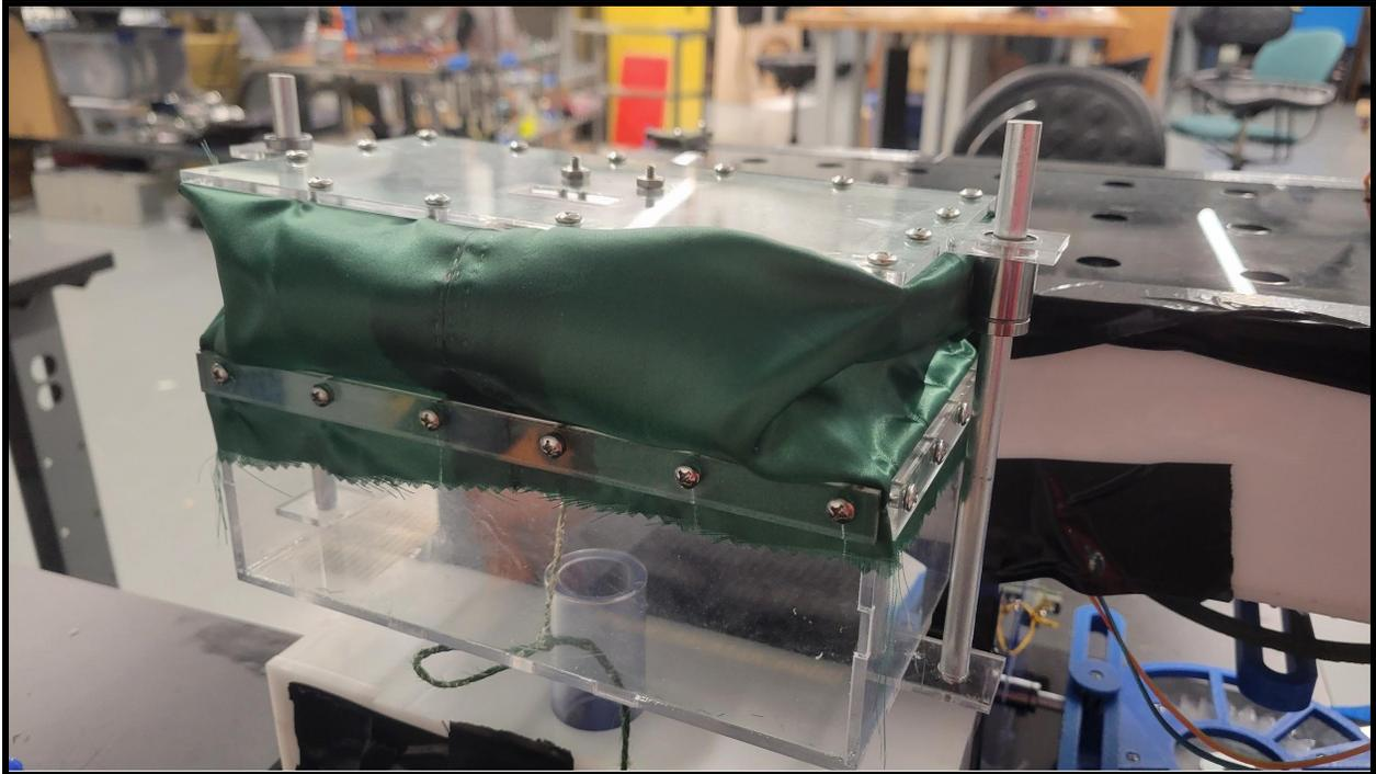
**Figure 19: Picture of the pressure regulator mounted on the organ. In normal operation, there would be a weight placed on the top to tune the pressure. Note the string going through the bottom that goes up to the valve.**
