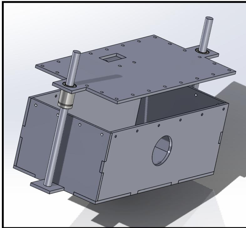
**Figure 18: Solidworks assembly of the pressure regulator. Note that neither the bellows or its mounting brackets are included.**
