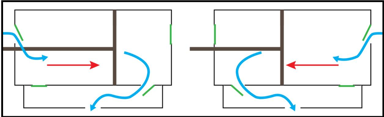
**Figure 13: Simple cross-sections of a typical box bellows design during the push stroke (left) and pull stroke (right). The blue arrows represent airflow, while the red arrow represents the piston's motion. The green lines represent one-way valves.**
