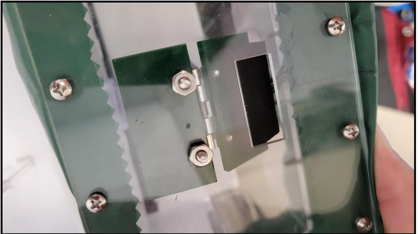
**Figure 20: Close-up picture of the top of the regulator, focusing on the open exhaust valve. Note the springed hinge.**
