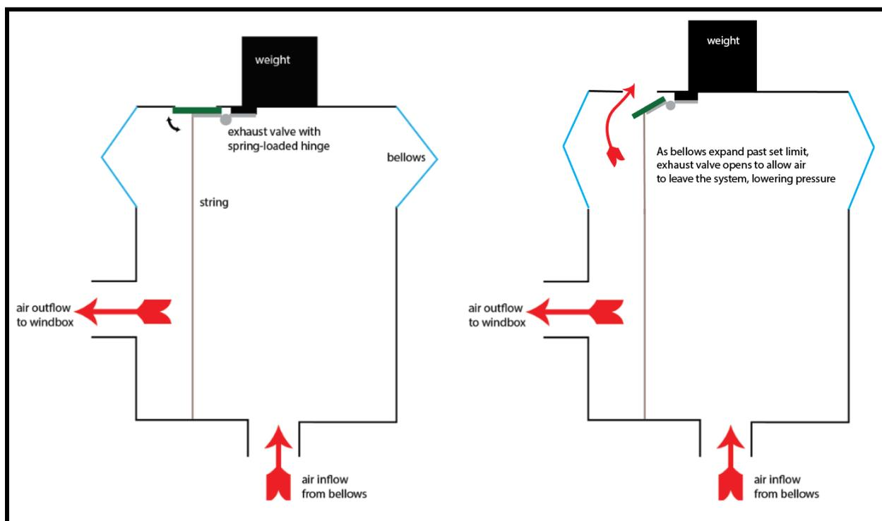
**Figure 17: Cross-sectional drawings of our pressure regulator operating at normal (left) and high pressure (right). Note the single compartment design, exhaust valve (open on the right to allow for the venting of excess pressure), and weight on top for tuning.**
