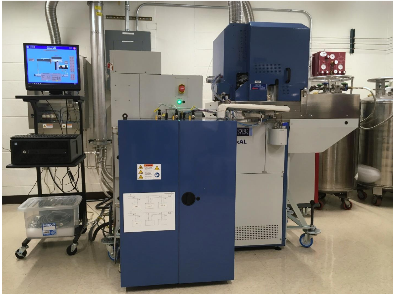
Figure 3.2: Oxford FlexAL II ALD system used for deposition of HZO thin films.
