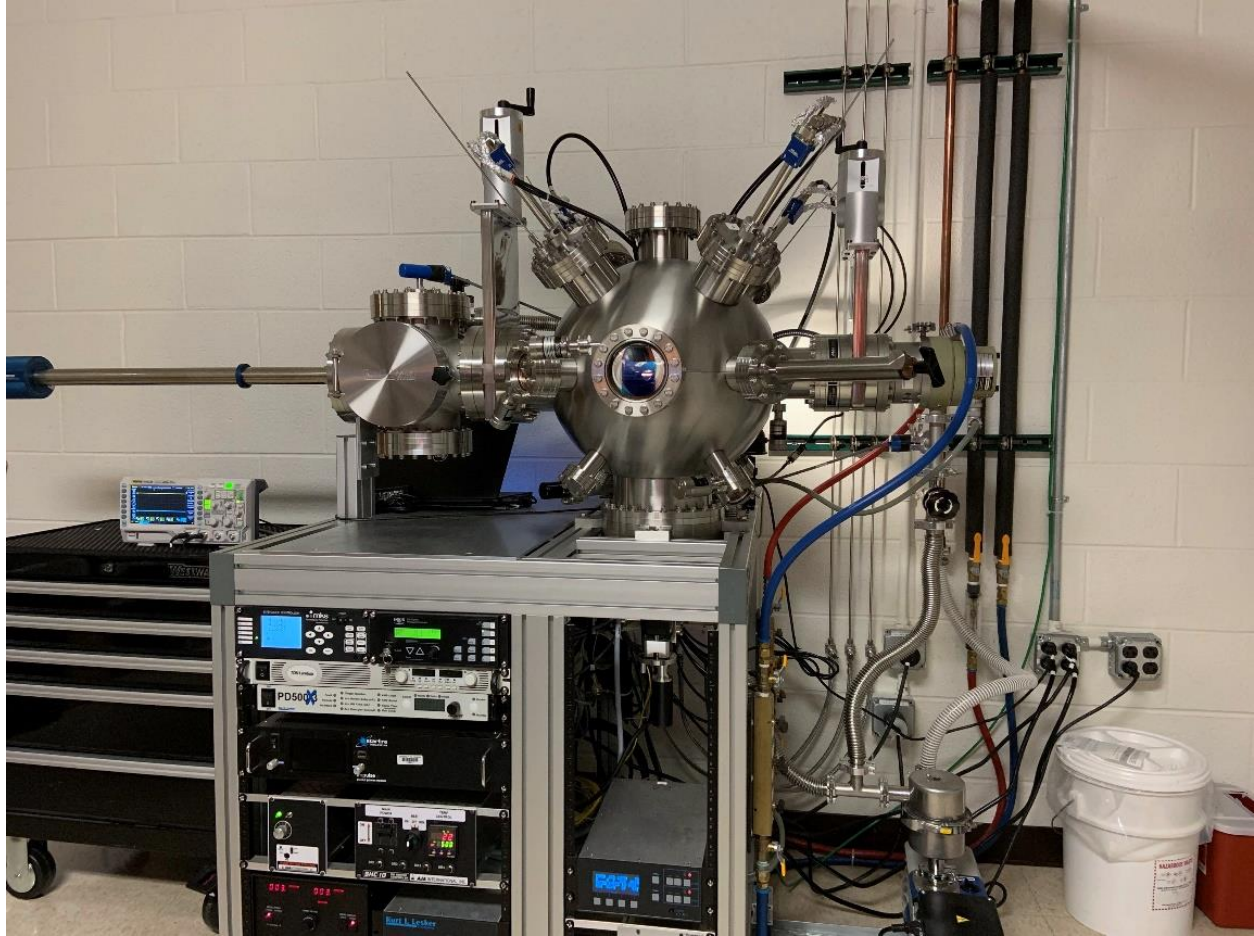
Figure 3.6: Sputter system used for HiPIMS depositions of \text{HfO}_2 -based thin films.
