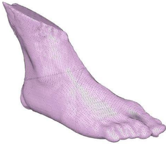
Figure 2: Sample 3D Foot Scan. 3D scan of a team member's foot obtained via photogrammetry and imported into Autodesk Fusion 360®. The 3D scan was used to create a contour body in the CAD workspace and imprint the topographical contours of the patient's plantar surface into the midsole body to achieve orthotic support throughout the midsole.
