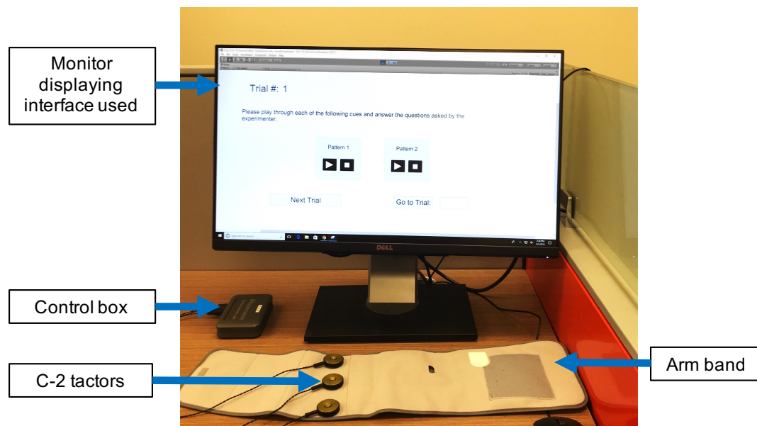
Figure 3.2 Tactile cue response task experimental setup including the interface participants used to play the tactile cues
