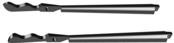
Fig. 2. Rendering of Final Device Iteration Used in Testing. The CAD rendering is of the final sinusoidal blade design that was printed in resin using an SLA printer and used in dry testing discussed in Materials and Methods.
