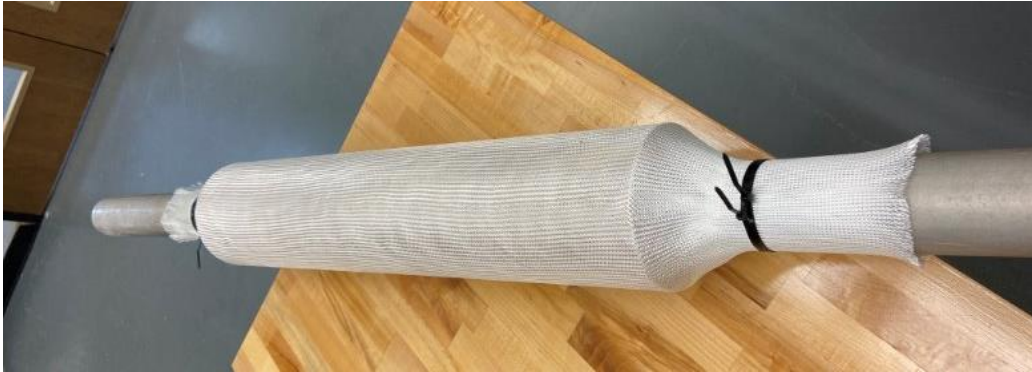
Figure 63. Fiberglass sleeve fixed over phenolic tubing.
