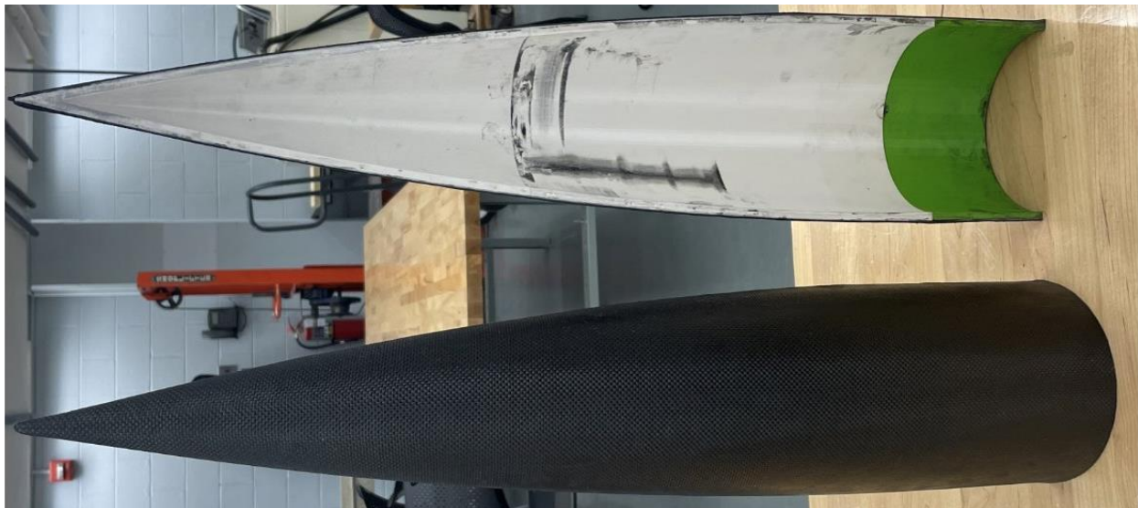
Figure 57. After 3 layers of CFRP wet layup
