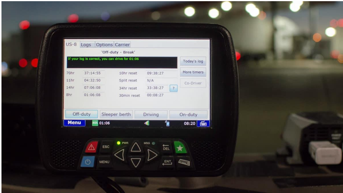
Figure 2: Picture of a system installed by companies into trucks to monitor the number of hours that have been drive. The system also displays how much longer a trucker can drive before they must take a break. (Gallagher, 2020, n.p.)
