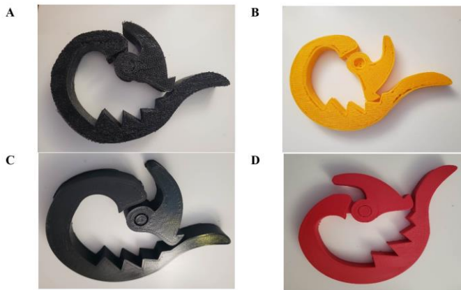
Fig. 4. Failed Tubing Clamp Prototypes. (A) Prototype A was printed with TPU in hopes that the flexible nature of the material would help it bend and secure the tubing more closely, but it was too spongy and not durable enough for its intended use. (B) Prototype B was printed with PLA but was too brittle due to too little infill density and was also too large, allowing the tubing to slip through. (C) Prototype C was printed with PLA and PVA supports, but the hinge had stuck together during printing, so the clamp could not close properly even though the PVA supports had entirely dissolved. (D) Prototype D was sized down again but still did not achieve the desired fit with all of the tubing, and the hinge had once again failed and broken off.
