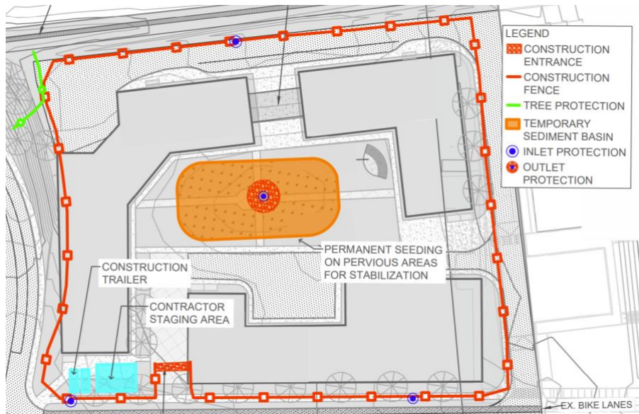
Figure 20. Phase II of the ESC plan. Bioretention serves as the sediment basin.
