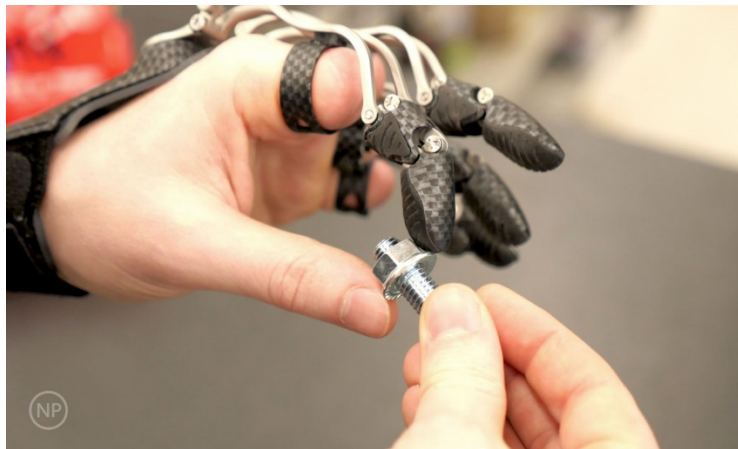
Figure 6. Naked Prosthetics finger prostheses with 3D printed componentry. Retrieved from https://www.pacerehab.com/news/naked/
