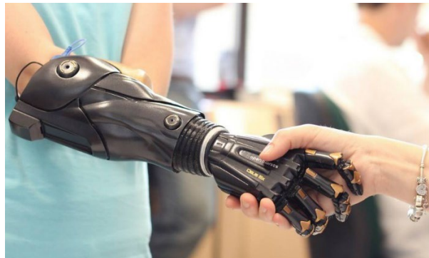
Figure 5. Open Bionics' 3D Printed Hero Arm. Retrieved from https://www.accessandmobilityprofessional.com/prosthetics-firm-targets-nhs-affordable-3d-printed-super-hero-arms/
