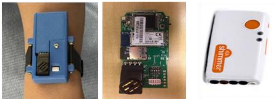
Figure 2.4: Custom designed wrist-worn device (left, center) to monitor pollutant concentration and sense wrist motion, Shimmer ECG sensing unit (right) is worn on chest to sense ambulatory ECG
