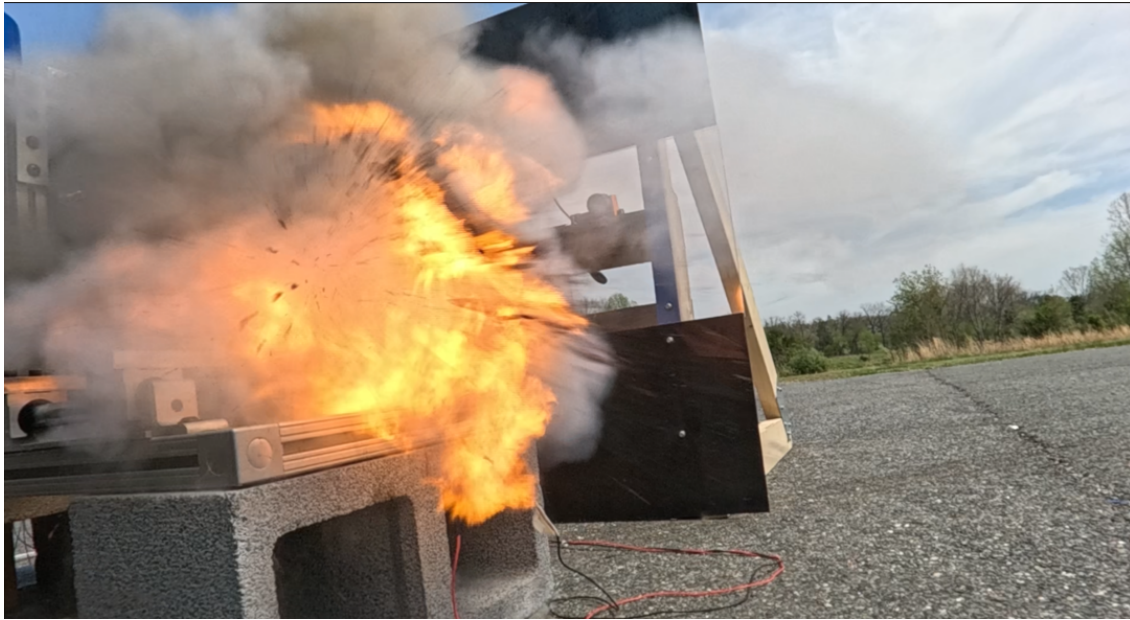
Figure 31: Failure of nozzle bulkhead during hot fire attempt four.
