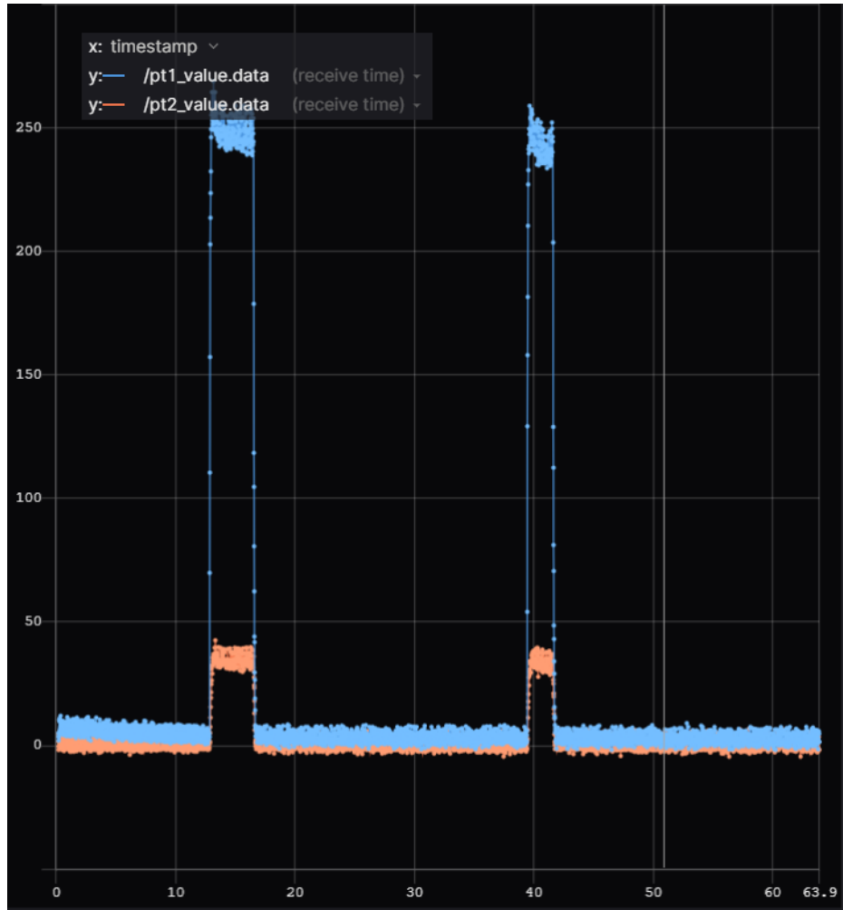
Figure 29: Pressure (psi) versus time (ms) data for cold flow test with needle valve at 50% open position.
