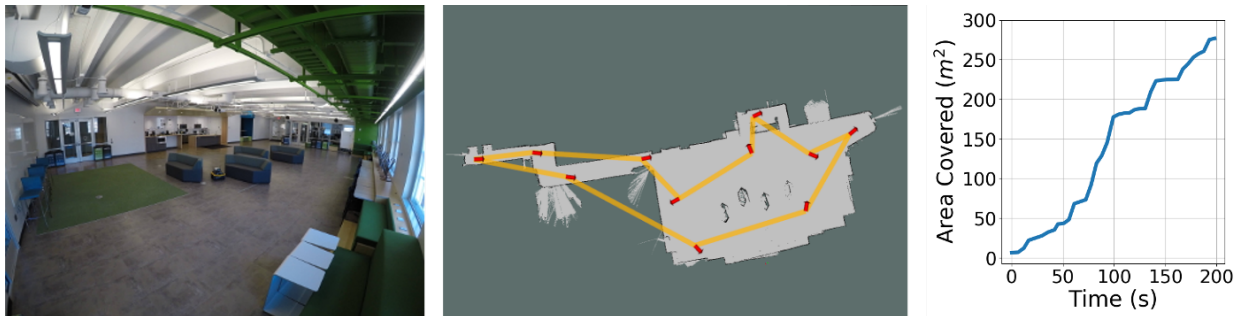
Figure 6.13: Office setup (left), associated map with watchman tour (middle), and coverage over time (right).
