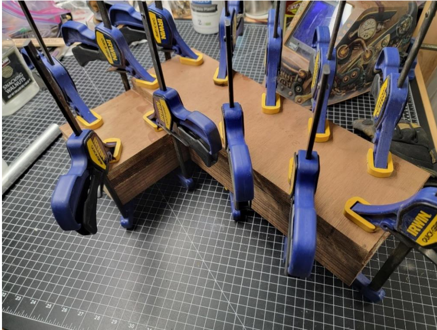
Fig. 3.3.4. Upper Playfield Plywood Stock Glued
