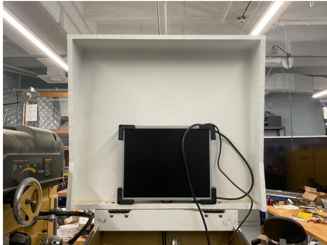
Fig. 3.6.1. Headboard of the pinball machine
