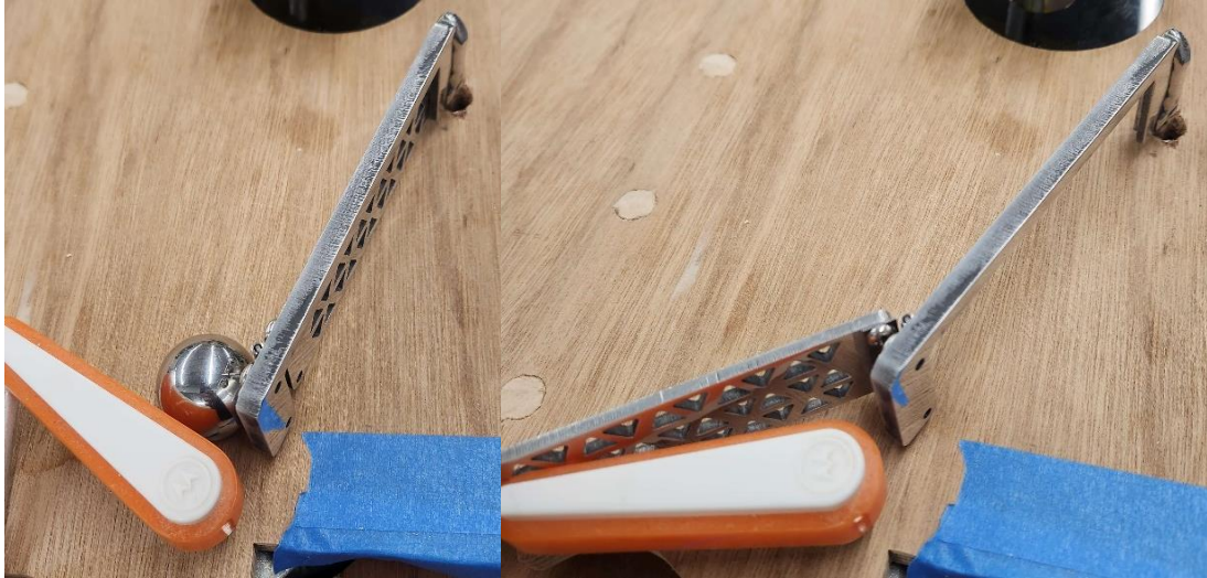
Fig. 2.5.1. Diverter gate illustrating the ability to hold a ball in place and illustrating the one-way gate functionality
