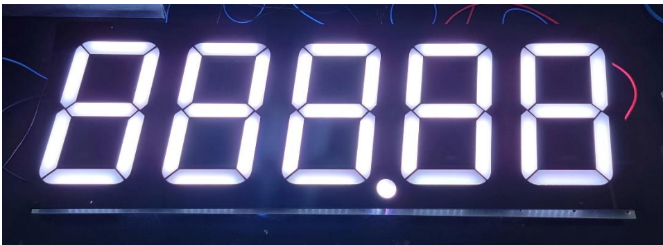
Fig. 2.10.7. Complete LED Backlit Acrylic
