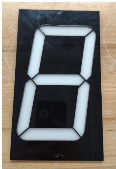
Fig. 2.10.1. Single acrylic digit prototype
