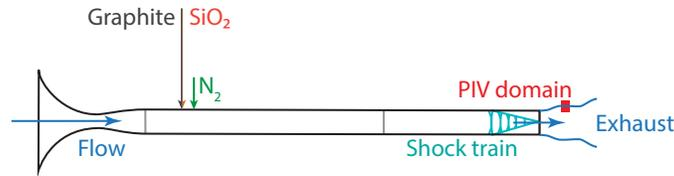
Figure 3.11: Schematic of the flow path and PIV field of view up to scale relative to the tunnel.
