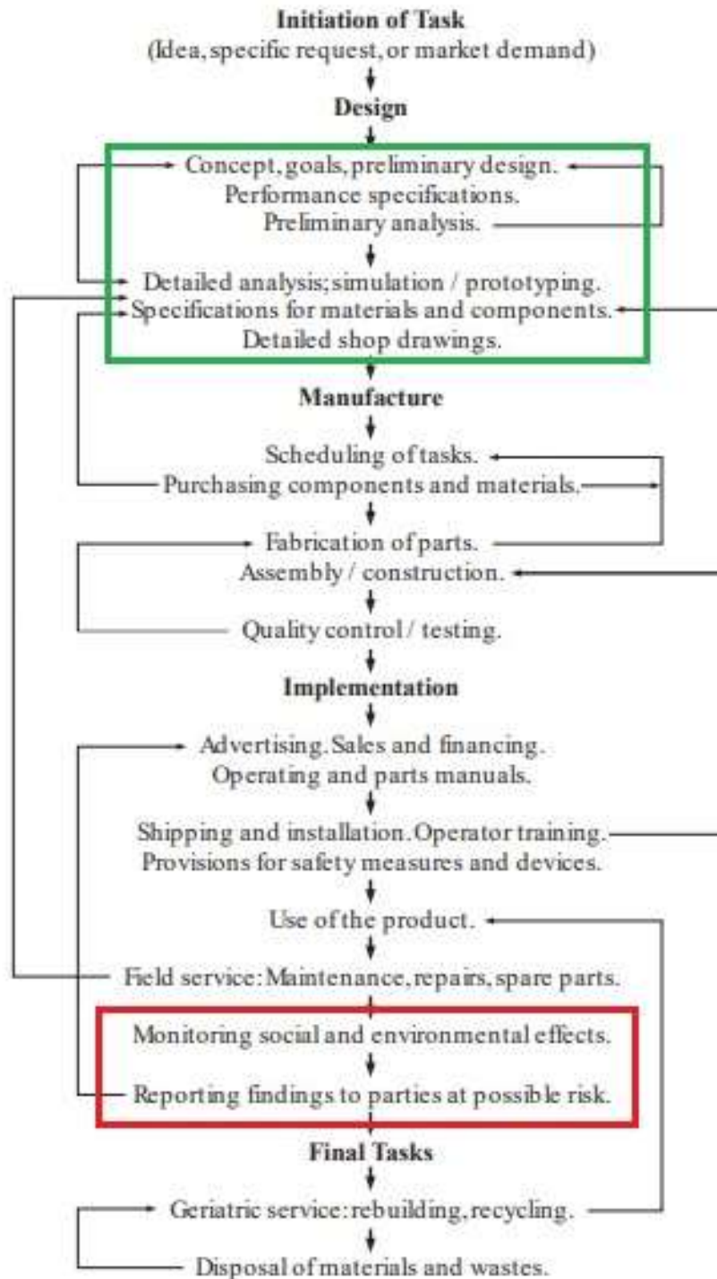
Figure 3: Current Progression of Engineering Tasks. Proposed national data privacy legislation could be implemented and further enforced through changes to the progression of engineering design and integration tasks. The tasks in red demonstrate the late consideration of social effects, while the tasks highlighted in green demonstrate a potential point much earlier in the process for incorporation of data privacy considerations to comply with proposed legislation (Adapted by Gustad, 2021, from Martin & Schinzing, 2009b).
