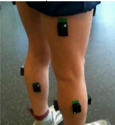
Figure 2: Sensor Example. An example of a set of Trigno sensors placed on a participant's Vastus lateralis and Bicep femoris. Each device contains an accelerometer, gyroscope, and EMG sensors (Hamrock, 2021).
