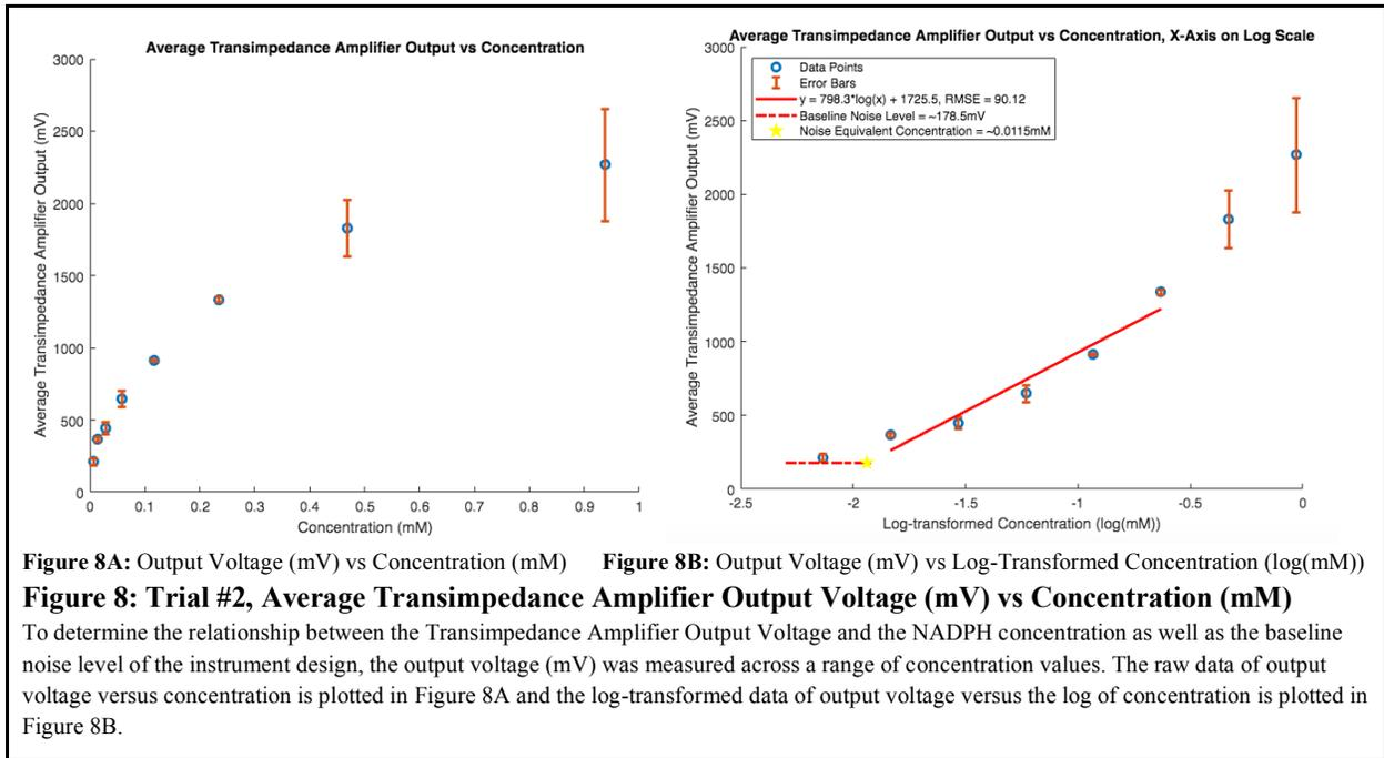
**Figure 8A:** Output Voltage (mV) vs Concentration (mM)    **Figure 8B:** Output Voltage (mV) vs Log-Transformed Concentration (log(mM))
