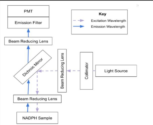
Figure 3: Instrument Optical Component Diagram
