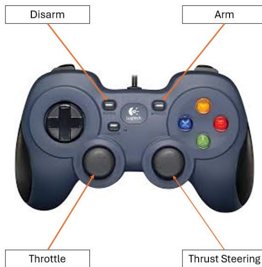
Figure 14: Mapping of Controls on Logitech Gamepad
