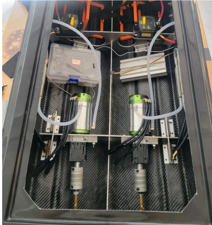
Figure 20: View of the Drivetrain and Navigation Systems
