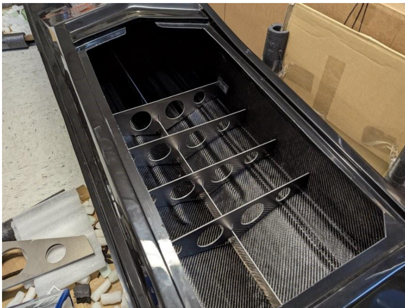
Figure 5: BSU, Shown Above from Water Jetted Aluminum, Inside the Hull
