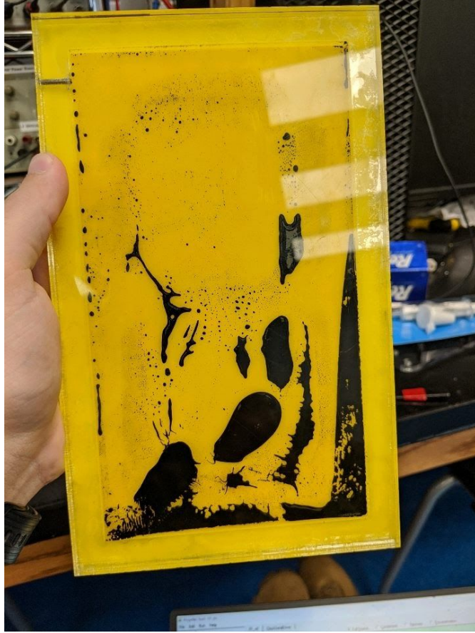
Figure 18: The coagulated ferrofluid inside of the acrylic tank
