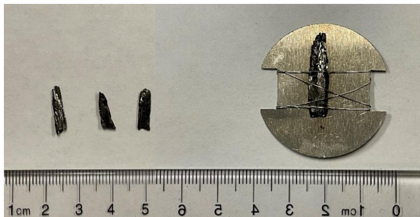
Fig. 4.1 Single crystals of \text{MoTe}_2 (three on the left) and \text{Mo}_{0.94}\text{W}_{0.06}\text{Te}_2 (the one on right, mounted on an aluminum plate).
