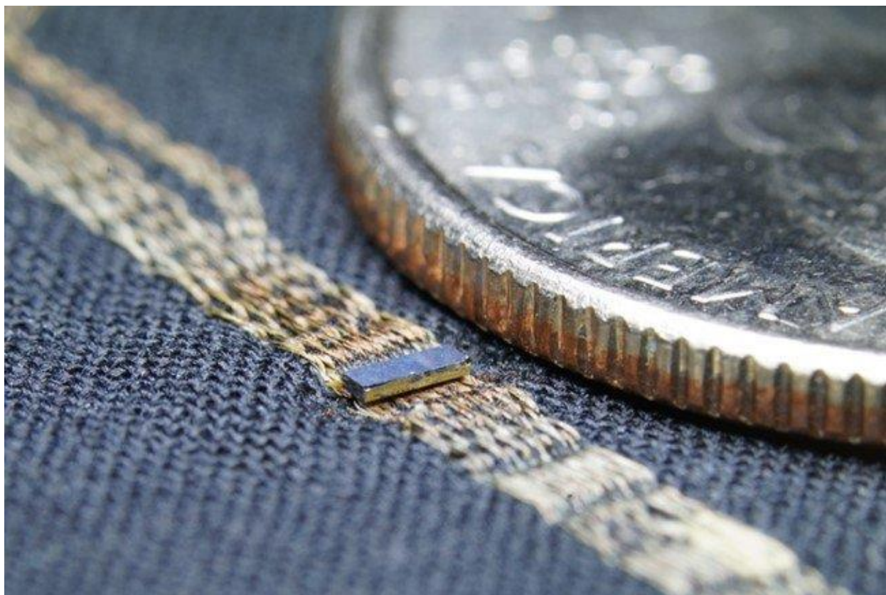
Figure 1. My team's networking chip attached to a fabric and positioned next to a dime.
