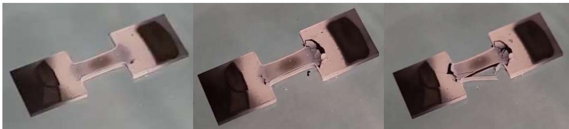
Figure 3.19: Time sequence of macro photos showing the spontaneous breakdown of the oxide scale formed on a single ZrC sample oxidized at 1400°C for 5 min in 1% O<sub>2</sub> – Ar. From left to right, the pictures show the sample 1 min, 3 min, and 5 min after being removed from the RHS.
