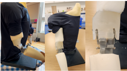
Fig. 5. Final prototype of joint reduction trainer. Final printed and cast elbow joint mechanism mounted to the shoulder and torso on a stand.
