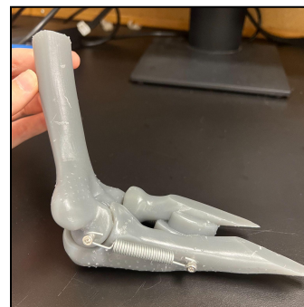
Figure 2: 3D-printed anatomically accurate elbow joint model
