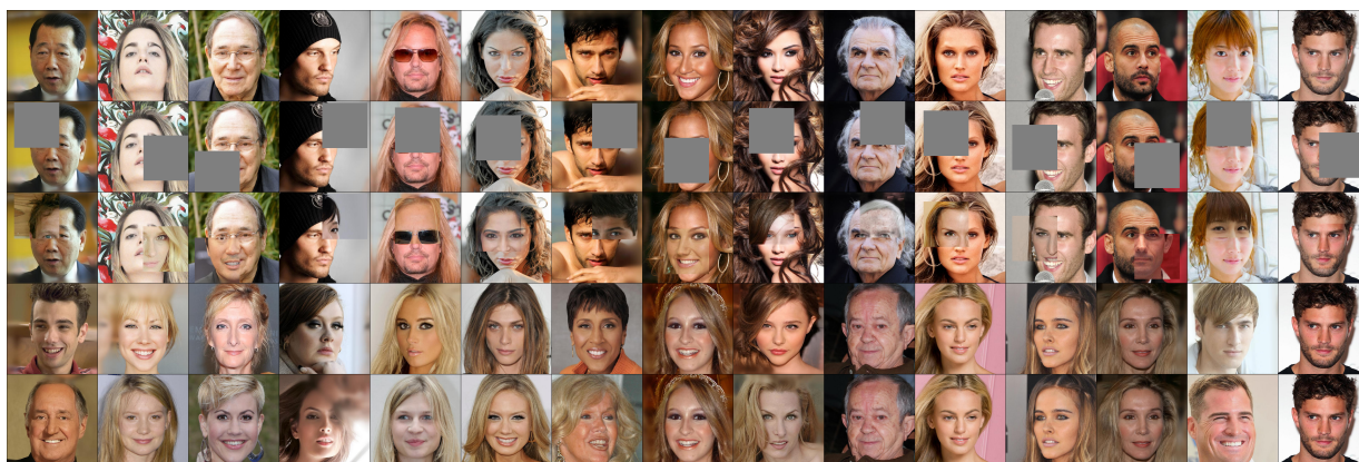
Figure 2.14: Inpainting result obtained with nearest neighbor (NN) search. 1st row: original image, 2nd row: occluded images, 3rd row: recovered images by NN search with the groundtruth patch, 4th row: recovered images by NN search with the original image, 5th row: recovered images by NN search using the occluded image. To perform inpainting with NN using the groundtruth patch, we search the dataset for the patch that has the minimum L_2 distance to the groundtruth patch, and then copy this patch to the occluded region.
