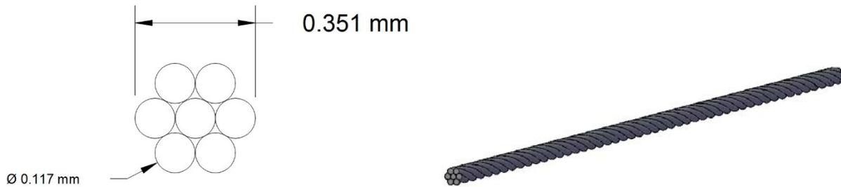
**Figure 4-1.** Cross-sectional and longitudinal view of SMA fibers
