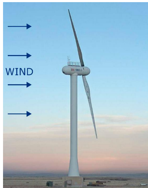
Figure 1-2. Downwind turbine schematic with wind direction shown for the SUMR-D rotor on CART-2 at the NREL Flatirons Campus outside Boulder, Co. (base webcam photo courtesy of Lee Jay Fingersh, NREL).
