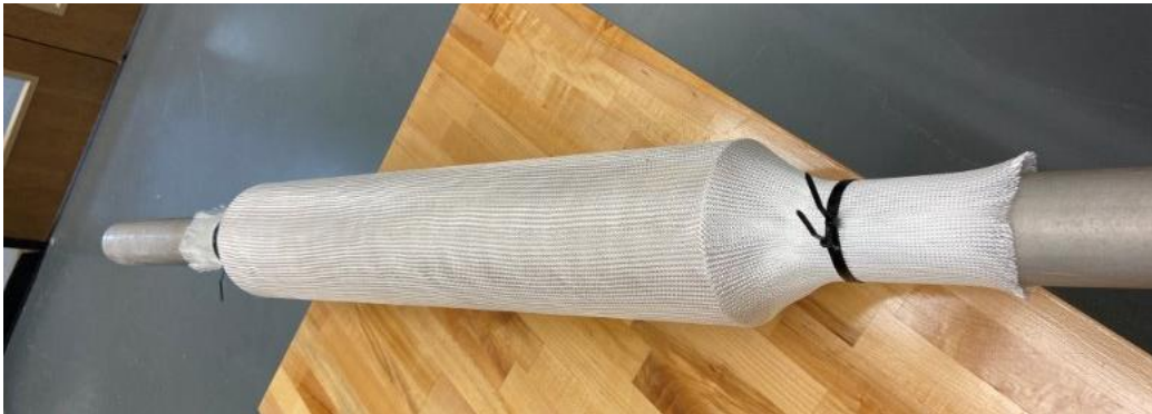
Figure 63. Fiberglass sleeve fixed over phenolic tubing.
