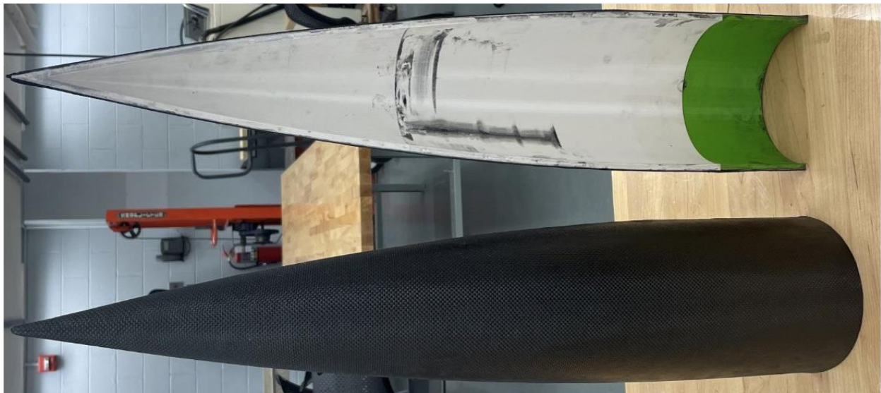
Figure 57. After 3 layers of CFRP wet layup
