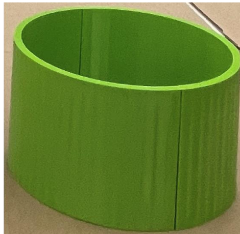
Figure 55. Extended nosecone mold (Height 10 cm)
