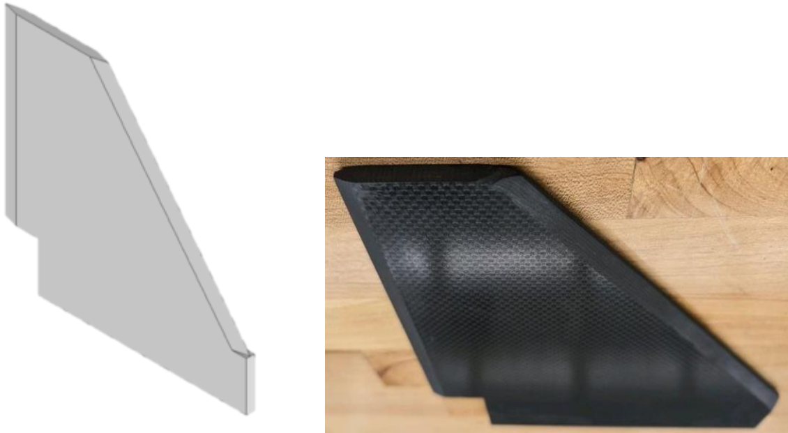
Figure 60. Designed vs actual sanded fin
