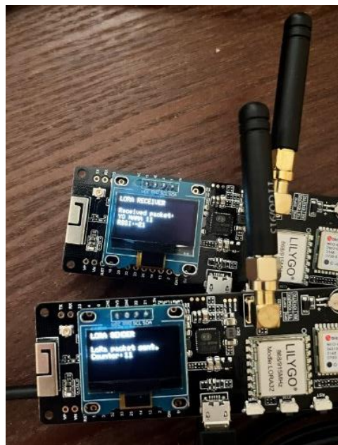
Figure 67. LCD of LoRa receiver module displaying static message (sender module's name) and dynamic message (number of packets sent by sender module)
