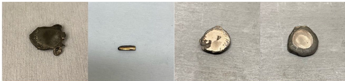
Ag 2 Yb ingot, bottom side, polished Ag 2 Yb after cutting inhomogeneous. Ag 2 Yb 3 ingot, bottom side, polished Ag 2 Yb 3 ingot, top side, polished
