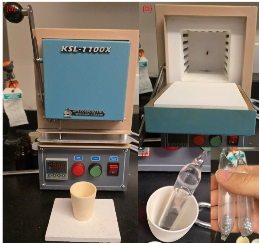
Figure 2-2 Muffle furnace and encapsulated ampoules. (a) muffle furnace (b) furnace chamber (c) encapsulated ampoule samples.
