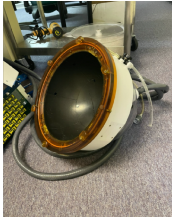
Fig. 3. The ExAblate Neuro Model 4000 Type 2 ultrasound transducer. This transducer has been developed by the medical device company known as Insightec, a company that sells MRgFUS equipment.
