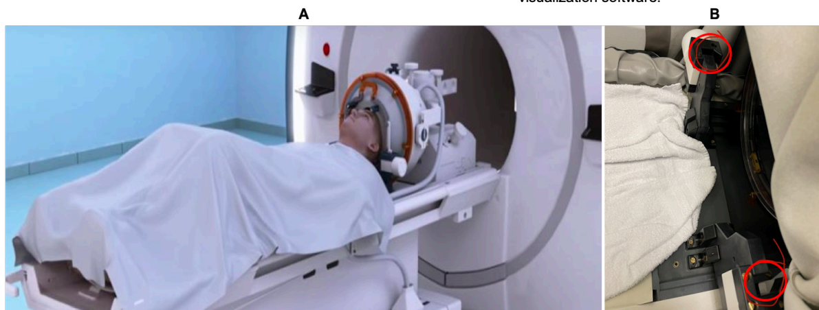
Fig. 4. Design Constraints. (A) A patient about to undergo a FUS procedure. The patient is fixed into position on the MRI bed with the headframe, which is interlocked into the FUS transducer. (B) The red circles highlight the mounting areas where the frame will have to attach prior to patient head fixation.
