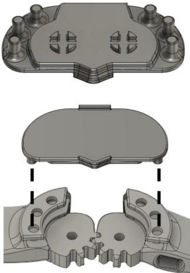
Figure 1. At the top we see the underside of the hinge cap that is then flipped over and guided into the gear housing which allows for complete inhibition of flexion and extension during initial stages of recovery of total knee replacements and ACL/MCL reconstructions.
