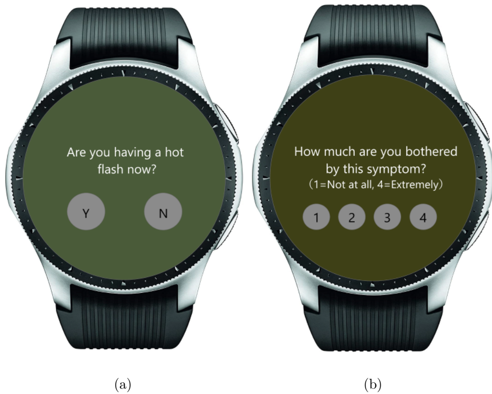
Figure 3.2: Smartwatch app prototype showing EMA survey about symptoms.
