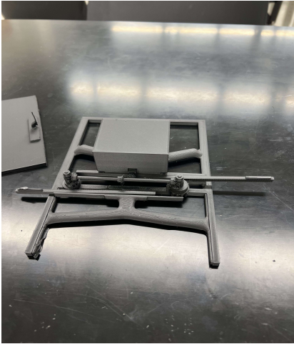
Fig. 4. Failed 3D model of design. First attempt at 3D printing the proposed design. Armrests snapped at attachment point due to excessive loading.
