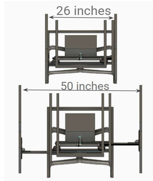
Fig. 3. Final CAD model of design. Isometric frontal point of view of final mechanism in retracted and expanded positions.
