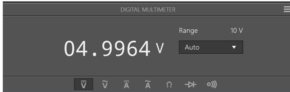
Figure 11: 5V Voltage Regulator Output
