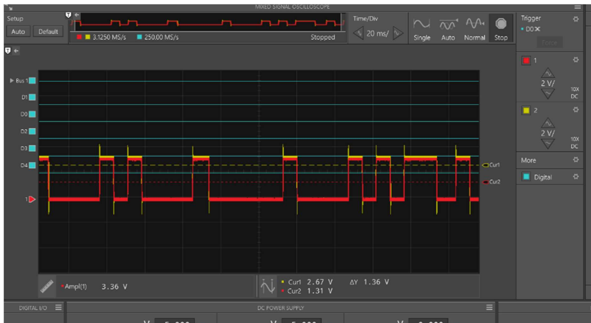
Figure 18: PWM Interrupts Varied Duty Cycle Test
