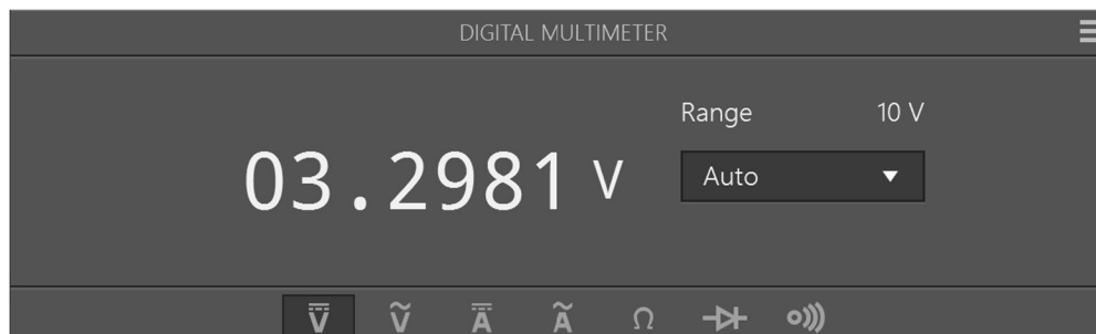
Figure 10: 3.3V Voltage Regulator Output
