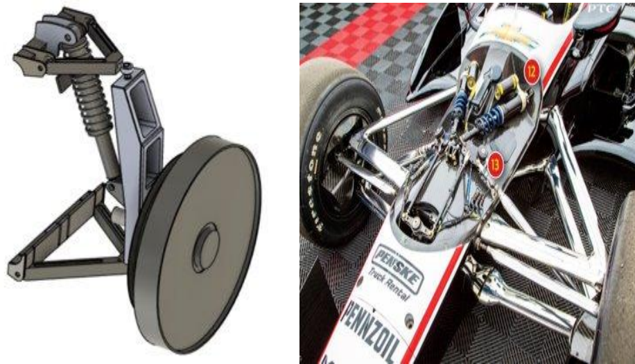
Figure 3: Rivanna 2 Solar car suspension (left) and Chevrolet IndyCar team pushrod suspension (right)
