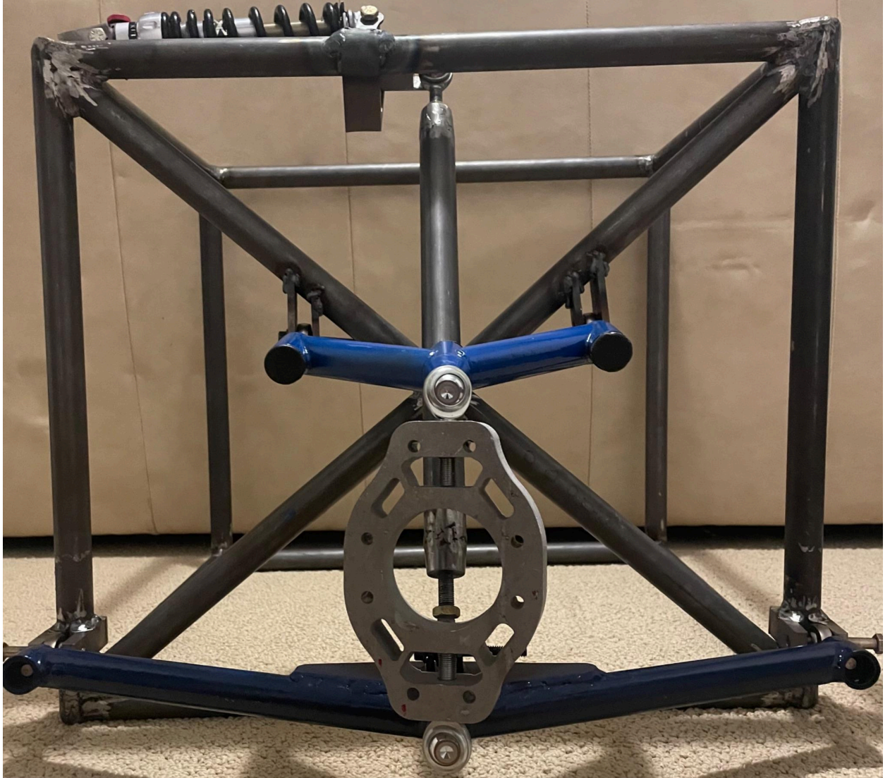
Figure 17: Front view of the suspension system. The upright has slots cut out to reduce weight
