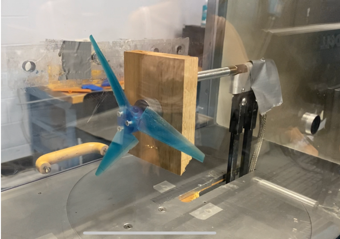
Figure 7. Testing apparatus with resin turbine secured with set screws
