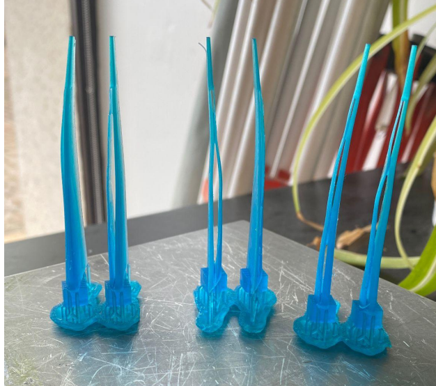
Figure 2. Resin blades after curing, seen with inconsistent forms across each blade type
