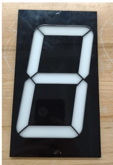
Fig. 2.10.1. Single acrylic digit prototype
