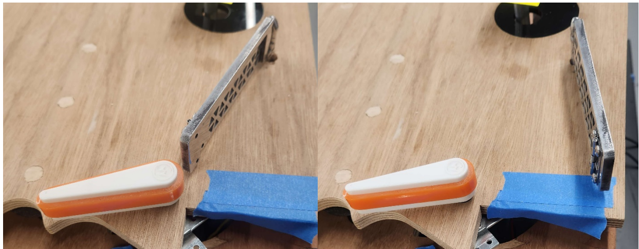
Fig. 2.5.2. Diverter gate in closed and open position
