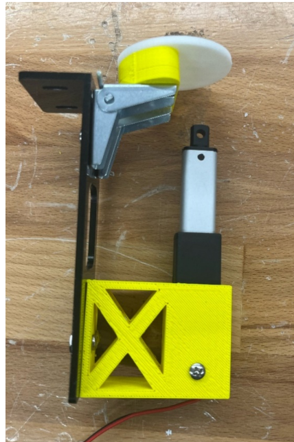
Fig. 2.6.3. First prototype of the vertical trapdoor design
