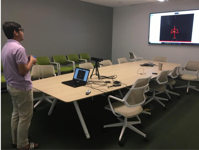
Figure 4.3: A subject playing the test corpus with a Bluetooth loudspeaker during Walk-Stop-and-Speak test.
