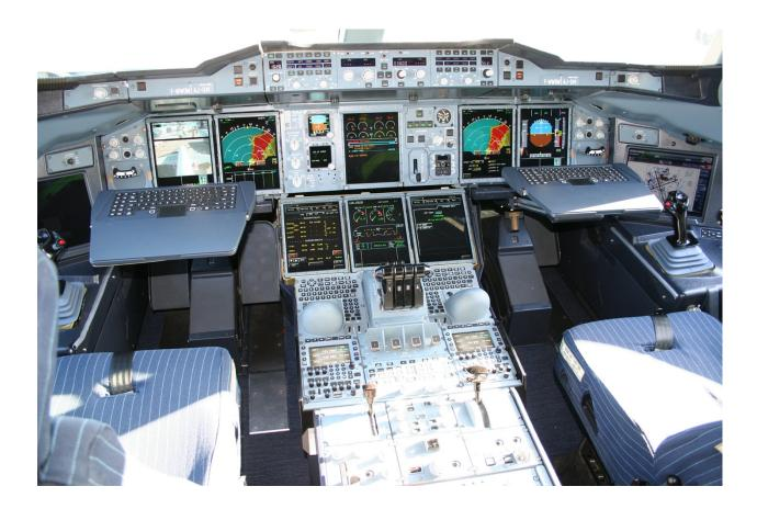
Figure 13. Side Sticks in an Airbus A380 Cockpit, Photo: Naddsy<sup>29</sup>
