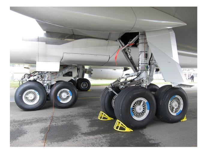
Figure 4. The Retractable Main Landing Gears on a Boeing 747, Photo: Olivier Cleynen<sup>20</sup>
