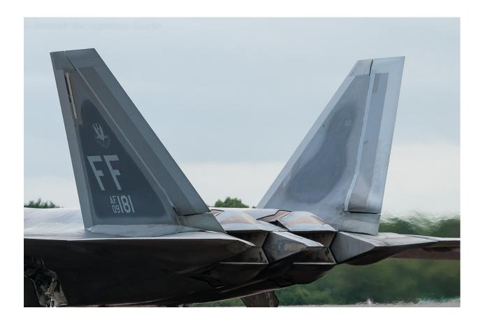
Figure 5. Angled Stabilizers on a Lockheed Martin F22, Photo: aircraftrecognitionguide.com<sup>21</sup>
