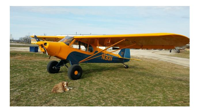
Figure 6. Large Diameter Tires on a Piper Cub, Photo: Steve Pierce<sup>22</sup>
