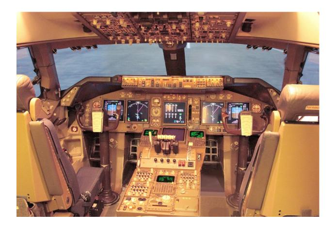
Figure 14. Center-Yokes in a Boeing 747 Cockpit, Photo: saitama<sup>30</sup>
