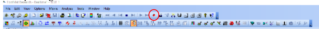
Figure C7.2.4. Tekscan screen highlighting where to click the “Record” button for the squatting trial
