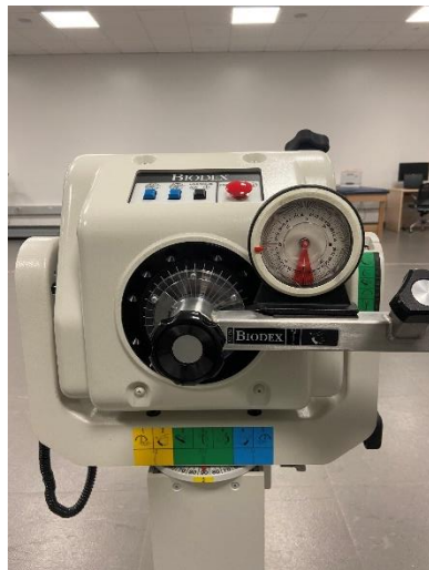
Figure C6.1.4.3. Biodex arm positioning to set the “AWAY” limit where the knee should be fully extended
