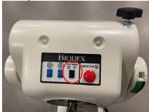
Figure C6.1.4.3.1. Biodex “Hold/Resume” button used to lock the arm in the current position.
