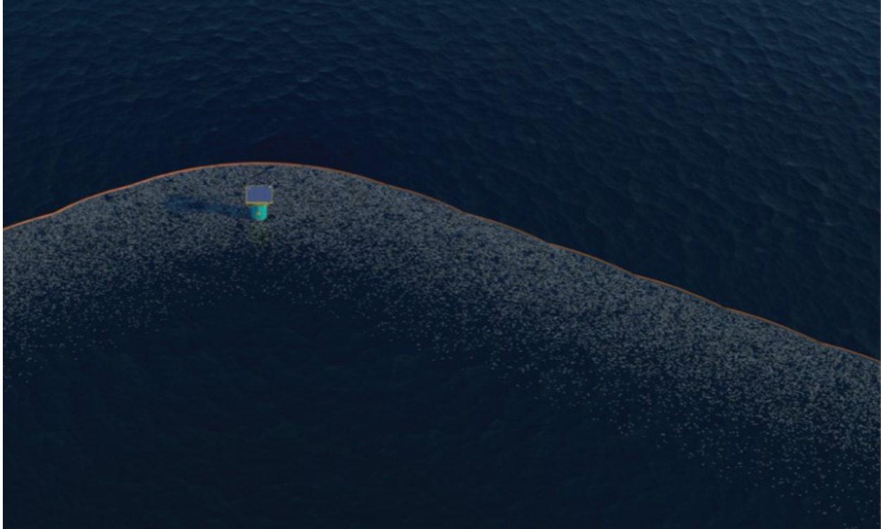
Figure 15. Proposed Ocean Cleanup Passive Collector (Slat, 2014). Image shows orange extended barriers funneling plastics towards the collection platform.
